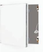
Removable door with 1/2" or 5%" drywall insert to blend in perfectly with walls or ceilings. Solidly built extruded aluminum frame and door. Nearly invisible 1/16" gap around door and frame. Gasket door perimeter adds resistance to air and smoke infiltration.
